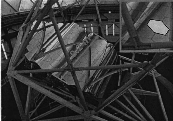
Figure 4. Segmented Primary Mirror of the Hobby-Eberly Telescope.
