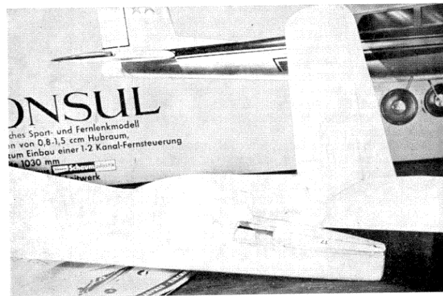
The vertical tail surfaces of "Consul" are balsa for the very good reason that there is no advantage in making them of E.P. They key into the moulded E.P. tailplane and are cemented permanently in place with PVA. Our preference is to do this before cementing the tailplane to the balsa platform on the rear fuselage, though the kit instructions reverse this order of assembly. Picture below shows the platform with a cutaway section for travel of the rudder push-rod which passes through an alloy tube.
